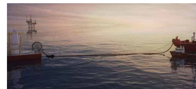
8. FPSO hawser and Offloading Hose connected...
