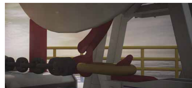
3. FPSO hawser Chafe Chain engaged...
