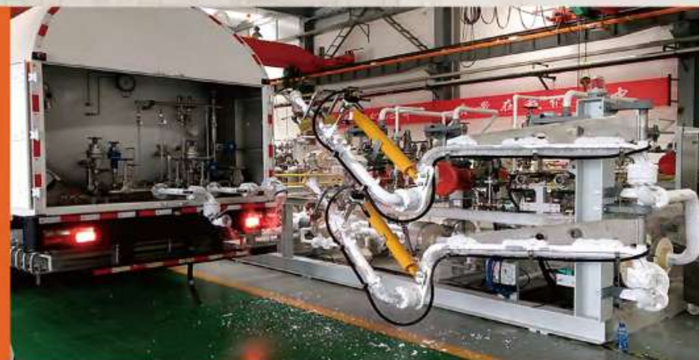
Cryogenic breakaway function test in CCLPEC workshop
